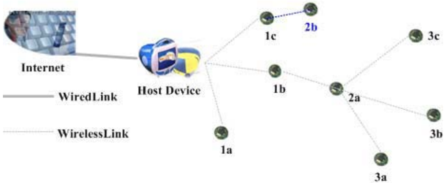
Fig. 3. Network topology reconstructs after a new mote (2b) was added
